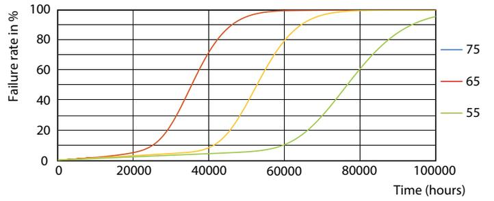
Lumen Maintenance Diagram - MAS LEDtube HF 1200mm HO 14W830 T8
